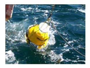
A "pop-up" listening device is deployed off the Massachusetts coast. The autonomous recording units listen for ocean noise from all sources 24/7. (Credit: Denise Risch, NEFSC/NOAA)
