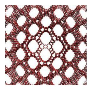
Zeolites are a fine lattice, a molecular sieve that can let molecules of a certain size pass while blocking others. Credit: Rice University
