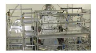
A scaffolding structure built around NASA's Wide-field Infrared Survey Explorer, or WISE, allows engineers to freeze its hydrogen coolant. The WISE infrared instrument is kept extremely cold by a bottle-like tank filled with frozen hydrogen, called the cryostat. The cryostat can be seen at the top of the spacecraft. Image credit: NASA/JPL-Caltech/Space Dynamics Lab
