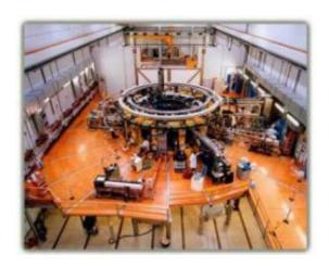
The RFX-mod Reversed Field Pinch (RFP) experiment has shown that higher currents lead to self-organized helical plasmas. Credit: Piero Martin, Padova, Italy
