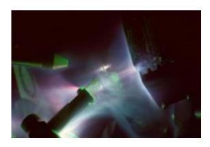
This is an image of the infrared laser (not seen, entering from left-hand side) interacting with a flat target (center), and the associated plasma production from the interaction on the various diagnostic instruments in the chamber. This is a time integrated image over five seconds. Credit: Joe Cowan and Kirk Flippo, LANL
