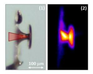
(1) Micro-scale Cu Flat-Top Cone target, with the incident laser (represented in red) coming from the left, (2) Cu K-alpha X-ray image showing the deep penetration of the laser light inside the cone neck.
