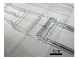
This photo shows a microinjection device loaded into a fixture which immobilizes the left substrate and ensures planar and linear motion of the movable substrate. Credit: McMaster Engineering
