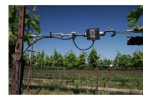
Trellis Tension Monitoring (TTM) assembly (center) in line with the main trellis wire in a wine grape vineyard. The row in the background also contains a TTM assembly (toward right). The metal post supports the vine at the left edge of the photo and is a normal part of this trellis system. Credit: Photo courtesy of Julie Tarara
