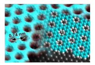
Scanning tunneling microscope image of the two-dimensional porous polymer (left side of image) with a model of the material structure superposed (right side: blue-green - carbon; white - hydrogen; gray - silver surface).
