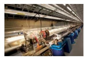
Thirty-three LCLS undulator magnets create intense X-ray laser light from a pulse of electrons traveling 99.9999999 percent the speed of light. Credit: Image courtesy of Brad Plummer, SLAC.
