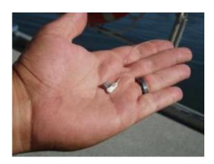
An acoustic tag (left) and a radio tag (white, with wires) sit in the palm of a researcher's hand. Both acoustic and radio tags are being implanted in juvenile fall Chinook salmon to track their movement at the confluence of the Clearwater and Snake rivers near Lewiston, Idaho. Credit: Pacific Northwest National Laboratory
