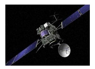
Artist view of ESA's Rosetta cometary probe. The spacecraft is covered with dark thermal insulation in order to keep its warmth while venturing into the coldness of the outer Solar System, beyond Mars orbit. Credits: ESA, image by AOES Medialab
