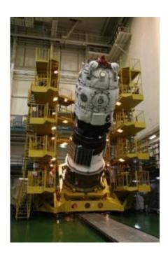
Scientists prepare the Mini-Research Module 2 (MRM 2) "Poisk" for flight at Kazakhstan's Baikonur cosmodrome on November 3. A Soyuz rocket carrying the new Russian-made module for the International Space Station blasted off from the Baikonur space base in Kazakhstan.
