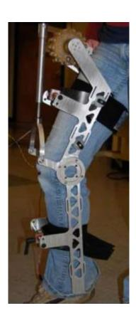
AKROD knee device from Northeastern University was designed to help a patient regain motor function after a stroke. The device is much smaller than similar systems currently in use. Credit: Biomedical Mechatronics Laboratory, Northeastern University
