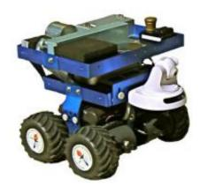
Cyclops is an all-wheel-drive platform that could enhance the design of visual prostheses and be adapted for autonomous planetary exploration. Credit: Caltech/Wolfgang Fink, Mark Tarbell
