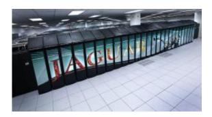
The Cray XT Jaguar features more than 224,000 processing cores, each with 2 gigabytes of local memory.
