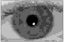
These compressed iris images from the IREX I test illustrate why the JPEG format did not meet the test criteria. The JPEG 2000 format (top) retains its quality after compression for storage and transmission, while the JPEG format (bottom) becomes pixilated when reduced the same amount. Credit: NIST
