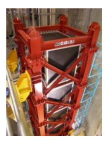
A photograph of the T2K INGRID neutrino detector. Each of the black cubes is a module of the INGRID.
