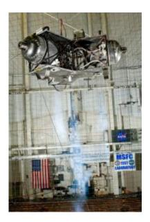
The robotic lunar lander test article is released from its hoist, while simultaneously receiving a command to activate it's onboard thrusters to carry it to a controlled landing using a pre-programmed descent profile. (NASA/MSFC/David Higginbotham)
