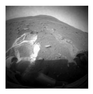
Wheel slippage during attempts to extricate NASA's Mars Rover Spirit from a patch of soft ground during the preceding two weeks had partially buried the wheels by the 1,899th Martian day, or sol, of the Spirit's mission on Mars (May 6, 2009). Image Credit: NASA/JPL-Caltech
