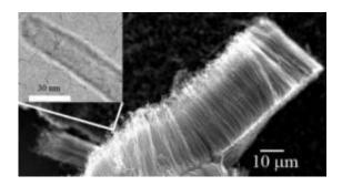
Carbon nanotubes could serve as supercapacitor electrodes with enhanced charge and energy storage capacity (inset: a magnified view of a single carbon nanotube). Credit: UC San Diego
