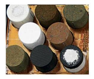
Samples of novel nanocomposite materials, seen above, will be mounted to the hull of the space station, and tested to see how they weather the perils of space.
