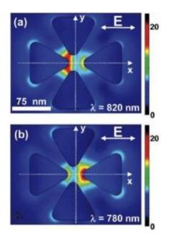
This scanning electron image of a nano color sorter with the vertical bowtie antenna shifted 5 nanometers (nm) to the left of center. In (a) the bowtie has been exited at 820 nm and in (b) at 780 nm. The two modes are spectrally and spatially distinct while maintaining nanoscale mode volumes. Credit: James Schuck, Berkeley Lab Molecular Foundry
