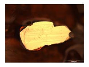
Image of the ferroelectric domains of the multiferroic compound BiFeO3. © A. Mougin, CNRS 2009
