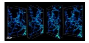
This image shows the 3-D nanoscale structure of the inside of a synthetic calcite crystal, which was grown in an agarose gel. In this environment, the crystal grows around the polymeric fibers. The structure gives insight into the formation of single crystals by biological organisms. Image: Estroff/Muller labs
