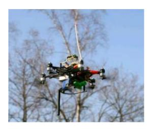
The MAV uses lasers and new algorithms to estimate its relative position, build a map, and locate a clear path. Image credit: MIT Robust Robotics Group.
