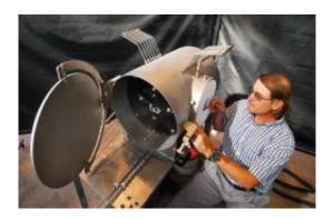
Sandia researcher Rich Diver assembles a prototype device intended to chemically reenergize carbon dioxide into carbon monoxide, which ultimately could become the building block to synthesize a liquid combustible fuel. Photo by Randy Montoya.
