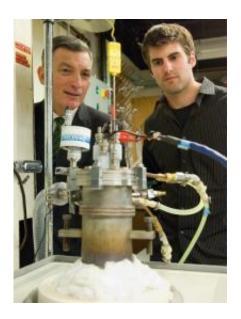
Professor Donald Sadoway and graduate student David Bradwell observe one of their small test batteries in the lab. The battery itself is inside the heavily insulated metal cylinder at center, which heats it to 700 degrees Celcius, while the wires at top charge up the battery and measure its performance. Photo: Patrick Gillooly
