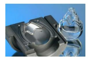
Metal mold for glass manufacture: the lower part of the mold has been left unprocessed, the upper part has been laser-polished. On the right, the product that can be made using a mold of this type. (© Fraunhofer ILT)
