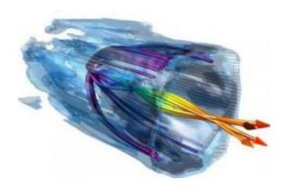
This is an example of a laser wakefield simulated in a "Boosted Frame." Electrons (colored tubes) are injected and accelerated by surfing the wave (blue surfaces) generated by a laser pulse. Credit: Samuel F. Martins, Instituto Superior Técnico
