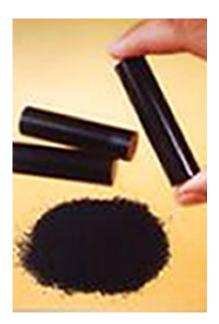
The two-inch fuel compact contains thousands of tiny particles of fuel.
