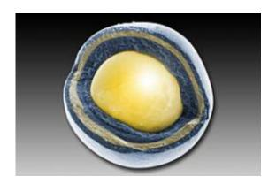
Each fuel particle contains a kernel of enriched uranium surrounded by carbon and carbide layers that act as containment boundaries for the radioactive material.
