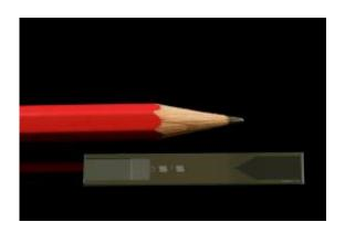
IBM Research scientists in Zurich have created a one-step point-of-care-diagnostic test, based on an innovative silicon chip that requires less sample volume, is significantly faster, portable, easy to use and can test for many diseases, including one of world's leading cause of death, cardiovascular disease. The chip in this photo measures 1 cm x 5 cm or 0.39 x 2 inches. Photo credit Michael Lowry, IBM Research
