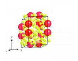
This schematic shows the structure of the new material, Xe(H2)7. Freely rotating hydrogen molecules (red dumbbells) surround xenon atoms (yellow). Credit: *Nature Chemistry*
