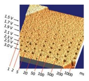
The surface morphology of modified Nb:STO surfaces. By using different electric pulse conditions, holes of different sizes and depths are created on a ~500-nm atomic-flat terrace. The sizes of the holes are ~10 to ~20 nm.
