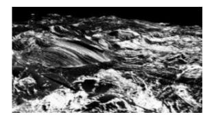
TOBI sidescan sonar imagery draped over multibeam bathymetry provides a unique 3-D view of an active oceanic core complex at 13°19'N, the Mid-Atlantic Ridge. The core complex is the smooth, striated dome forming the left-hand side of the image. To its right is the hummocky neovolcanic zone where recent volcanoes erupt lavas forming the the new oceanic crust. The field of view is around 30km wide. Credit: NOCS
