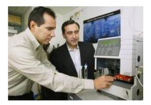
Biologist Benjamin Garcia (left) and chemical engineer Christodoulos Floudas collaborated to develop a fast and sensitive way to analyze proteins called histones, which play a key role in how genes function. Here, they load samples into a mass spectrometer, which separates and sequences hundreds of modified forms of histones. The work ultimately may aid the development of technology for reprogramming cells to fight cancer or to regenerate damaged tissue. (Photo: Frank Wojciechowski)
