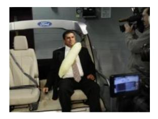
Ford's inflatable seat belts are designed for the rear seat. Image credit: Ford
