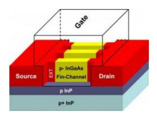
Researchers are making progress in developing new types of transistors, called finFETs, which use a finlike structure instead of the conventional flat design, possibly enabling engineers to create faster and more compact circuits and computer chips. The fins are made not of silicon, but from a material called indium-gallium-arsenide, as shown in this illustration. Credit: Birck Nanotechnology Center, Purdue University
