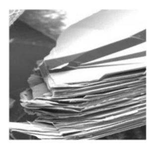
Graphene layers are found in graphite flakes like those from pencil lead. Image: Kirill Bolotkin
