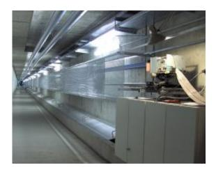
In a measurement channel the laser radar (on the right) determines the distance of an object up to 80 meters away every two microseconds or faster. (© Fraunhofer IPM)
