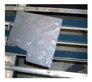
Solar wafers are only 150 to 180 micrometers thick, which makes them extremely delicate and fragile. (© Fraunhofer IPA)
