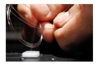
This close-up shows the brown light-absorbing material for the threedimensional solar cell grown on optical fiber by researchers at the Georgia Institute of Technology. Credit: Georgia Tech Photo: Gary Meek
