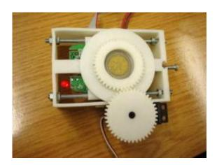
This image shows the detection of a false two-euro coin (this is a Thai currency) and detail of the optical sensor with a valid currency. Credit: Photos: Tresanchez et al. / SINC
