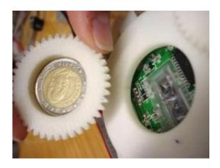
This image shows the detection of a false two-euro coin (this is a Thai currency) and detail of the optical sensor with a valid currency. Credit: Photo: Tresanchez et al. / SINC
