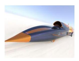
(PhysOrg.com) -- A British team hoping to be the first to get a car to 1,000 mph (1,610 km/h) has made its final design selection. The sixtonne car, known as the Bloodhound, will be powered by a Eurofighter jet engine mounted above a hybrid rocket, and will be built in Bristol, UK.
