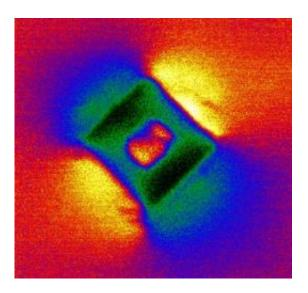
An image taken using polarized light microscopy. Clayton Lapointe, Thomas G. Mason and Ivan Smalyukh have succeeded in getting custom-shaped particles to interact and assemble in a controlled way in a liquid crystal. The colors indicate the direction of alignment of rod-like molecules outside the square microparticle. Credit: Clayton Lapointe/UCLA Chemistry and Physics
