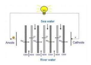
The principle of generating blue energy by reverse electrodialysis.
