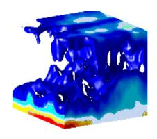
This image shows the 3-D concentration distribution of swimming bacteria Bacillus subtilis in thin liquid film obtained by optical coherence tomography.
