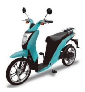
The Japanese electric zero-emission hybrid scooter "Miletto" to be released in 2010, which runs 10 times as economically as a petrol-engine bike and can be assisted by human pedal power, at the Prostaff company headquarters in Ichinomiya, Aichi prefecture, central Japan. The Miletto normally runs with battery power, but on a steep hill the rider would work the pedals to assist power.
