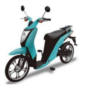
The Japanese electric zero-emission hybrid scooter "Miletto" to be released in 2010, which runs 10 times as economically as a petrol-engine bike and can be assisted by human pedal power, at the Prostaff company headquarters in Ichinomiya, Aichi prefecture, central Japan. The Miletto normally runs with battery power, but on a steep hill the rider would work the pedals to assist power.
