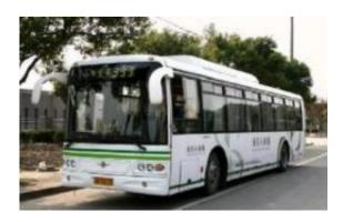
Buses with ultracapacitors stop at recharging stations, which double as bus stops, to recharge in less than a minute. Image credit: Sinautec.
