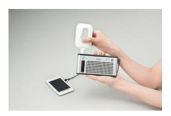
Dynario integrates Toshiba's state-of-the-art fuel cell technology, allowing it to operate with only a small volume of concentrated methanol solution, reducing the size and weight of the fuel tank and the overall
