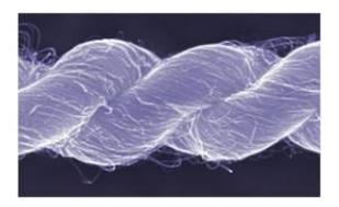
Wires made up of yarns spun from millions of carbon nanotube bundles may help make superconductivity practical. The nanofibers making up the wire are each thousands of times smaller than a human hair.
